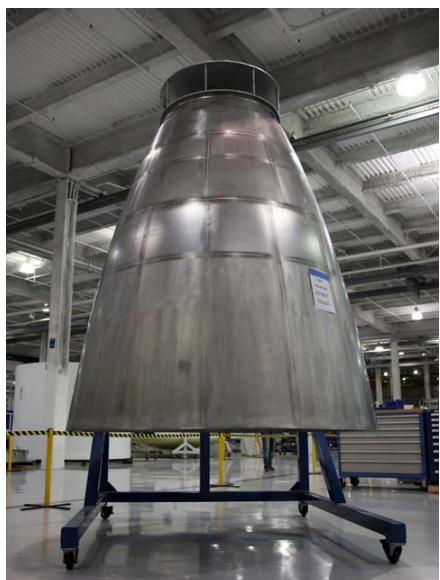
The Merlin Vacuum engine expansion nozzle, used on the second stage, measures 9 feet tall.
